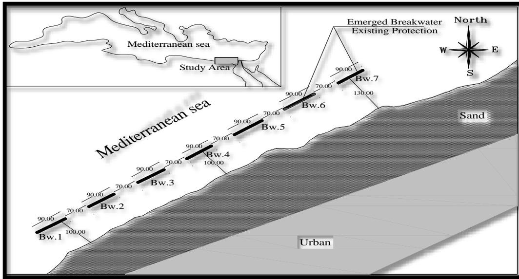
**Figure 2: The details of the breakwaters (Iskander et al., 2007, El-Kolfat A.Is, 2010), Drawing by the author**
