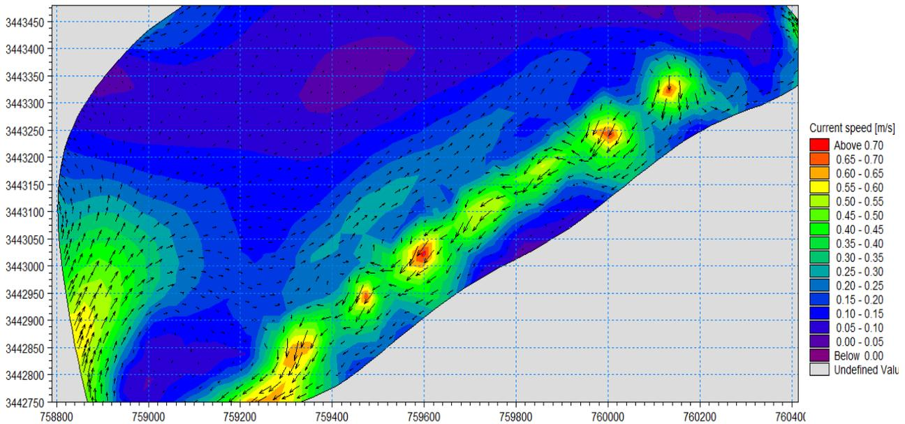
**Figure 11: Current direction and velocity for the seven submerged breakwaters.**
