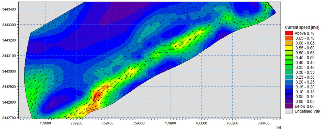
**Figure 14: Current direction and velocity for the 2 submerged breakwaters.**
