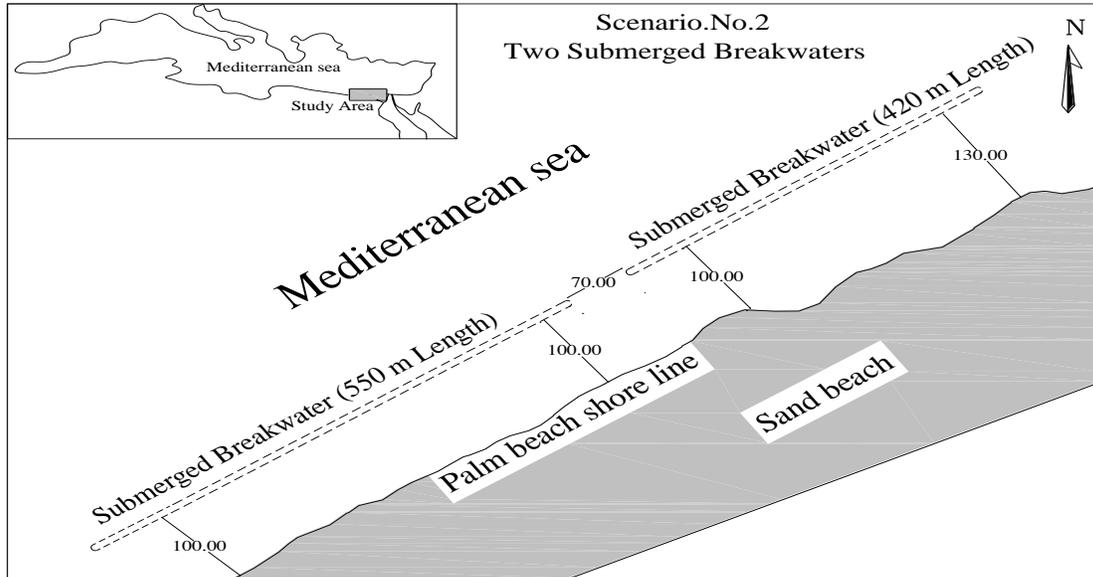
**Figure 12: The second scenario (Two submerged breakwaters)**
