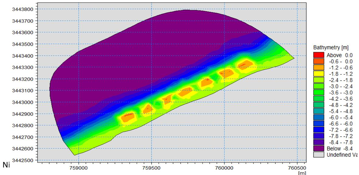
**Figure 10: The bathymetry of palm beach by Mike Zero for the 7 submerged breakwaters.**
