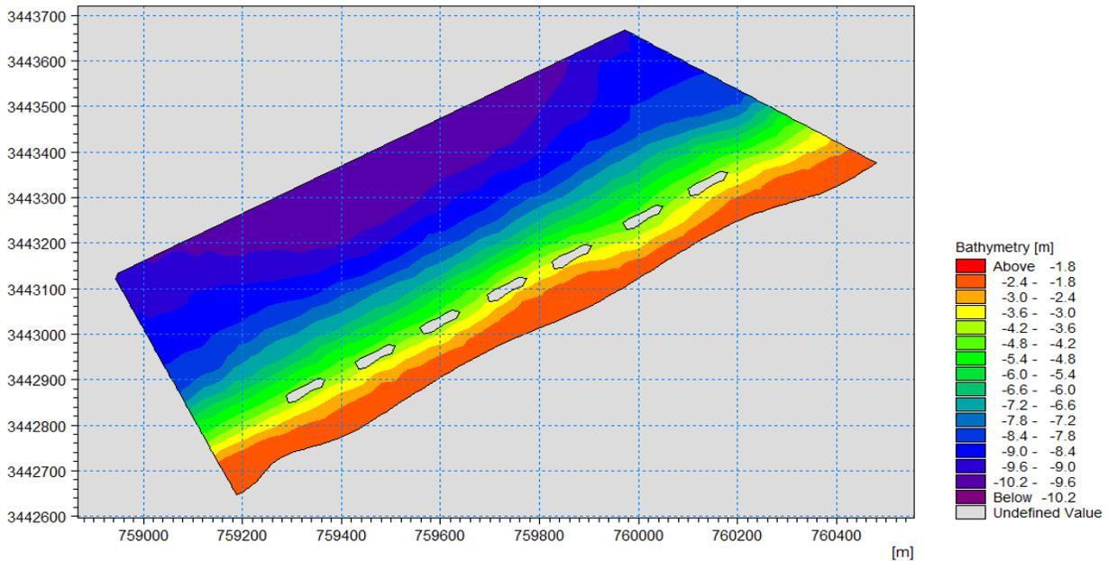
**Figure 8: The bathymetry of palm beach by mike 21 for the existing breakwaters.**
