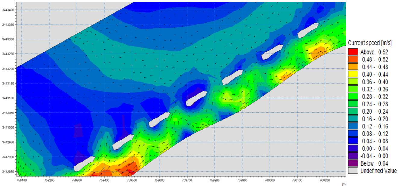
**Figure 9: The first scenario (Seven submerged breakwaters)**
