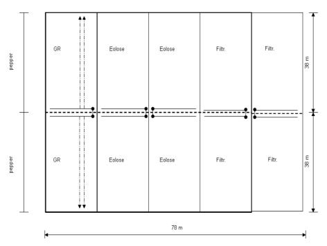
Figure 3: Irrigation setup in the greenhouse
