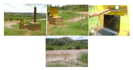
Figure 5: Gauging station installed at Rusumo for water level measurement of Kagera River.
