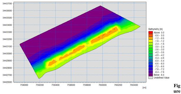
From mike zero we gain the new bathymetry of the first proposed solution as shown in Figure 13
