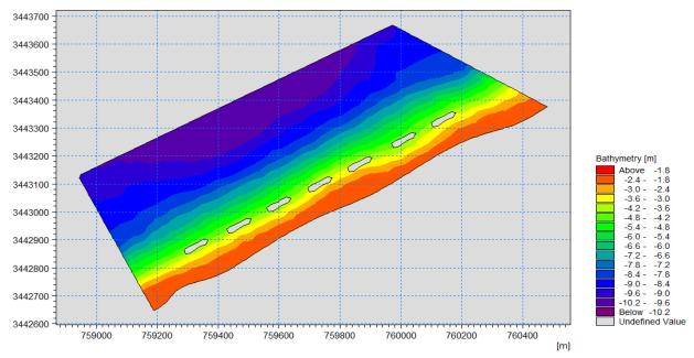
Figure 8: The bathymetry of palm beach by mike 21 for the existing breakwaters.
