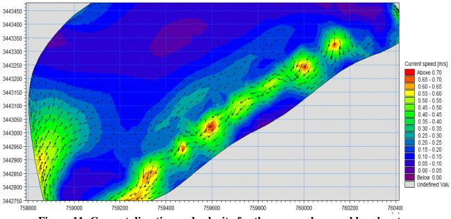
Figure 11: Current direction and velocity for the seven submerged breakwaters.
