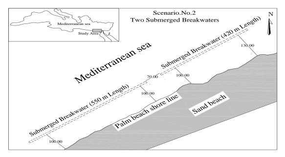
Figure 12: The second scenario (Two submerged breakwaters)
