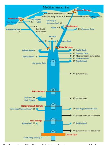
Figure 2: Pump Stations along Nile River (Ministry of water resources and irrigation, 2005)
