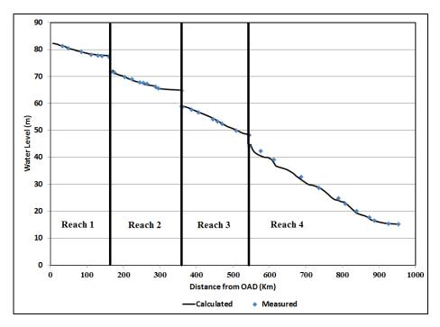
Figure 7: Model Calibration Results for first scenario
