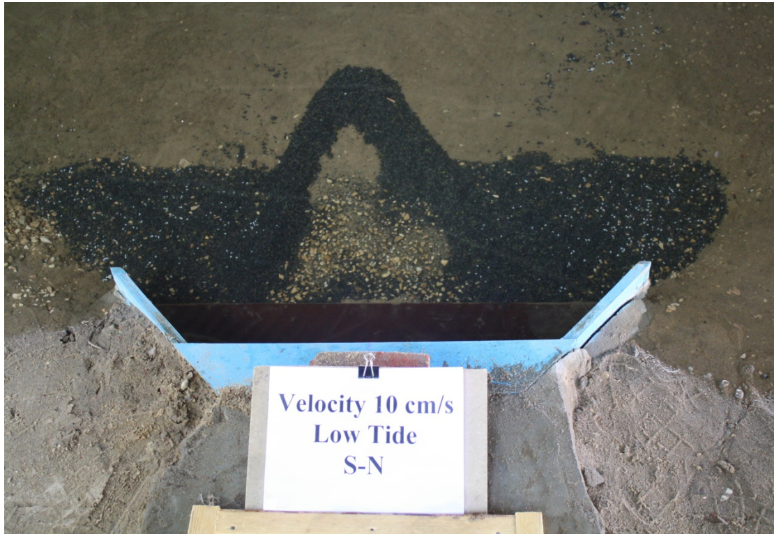
Figure 5: Erosion in the vicinity of the proposed outfall
