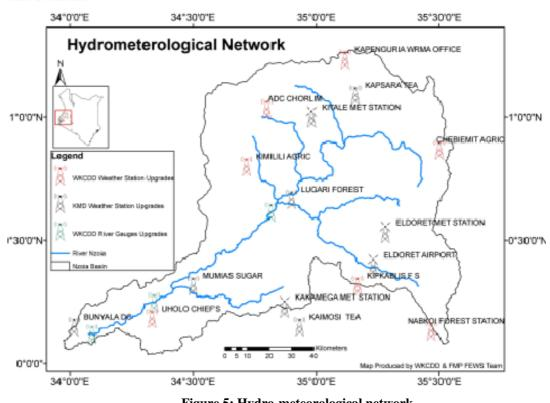
Figure 5: Hydro-meteorological network
