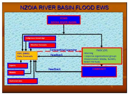
Figure 4: Early Warning System Components for Nzoia
