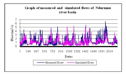
Figure 3: Measured and simulated flows of Ndurumu river basin
