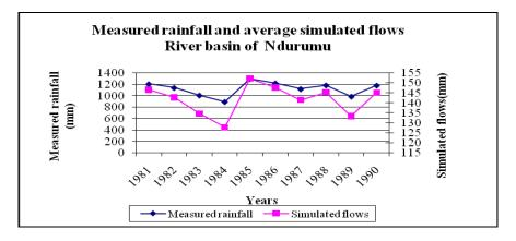
Figure 5: Measured rainfall and average simulated flows
