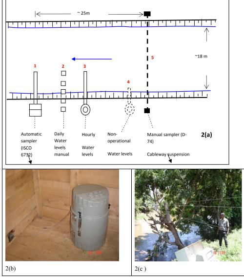
Fig. 2(a-c) Suspended sediment sampling equipment and layout design at the outlet of the test catchment 1DD1-Kikuletwa station.
