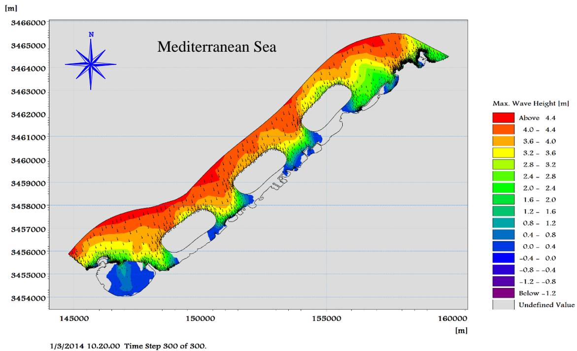
**Figure 14: Wave distribution by the annuals normal wave by max = 4.40 m**
