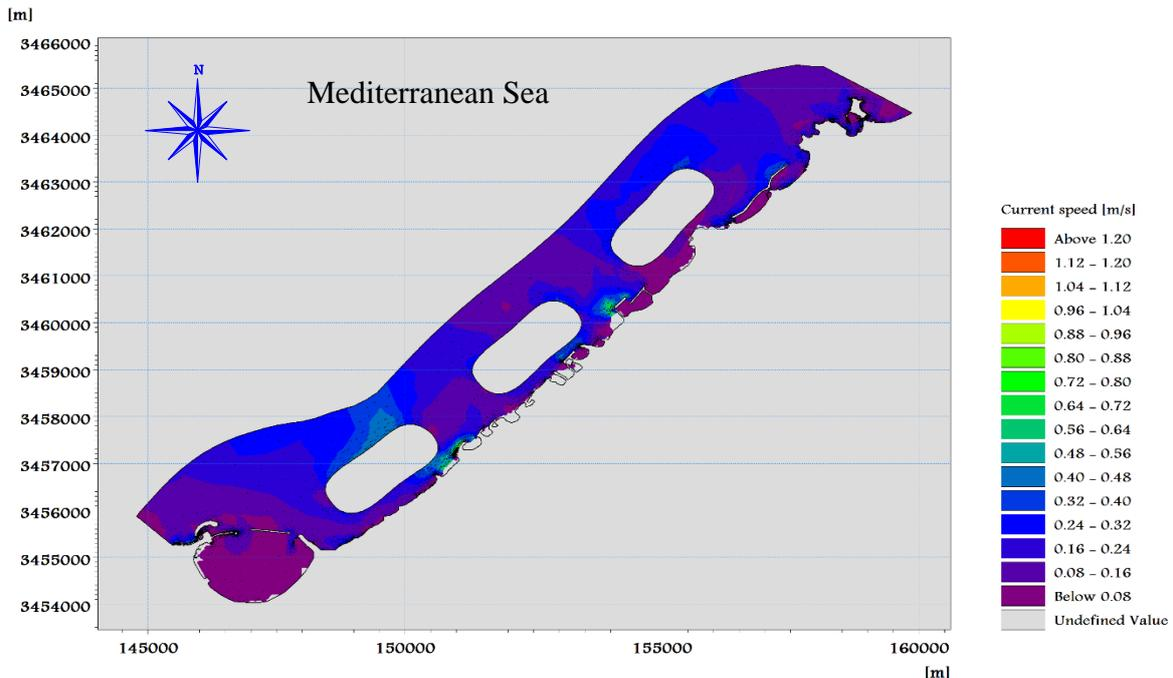
**Figure 15: current velocity distribution after constructing the islands which have a good swimming surf zone area**
