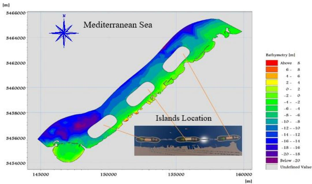
**Figure 9: Generated bathymetry by using Mike21 showed the different depths at the artificial island location. The end of the Artificial Island reaches a depth of 10 m.**
