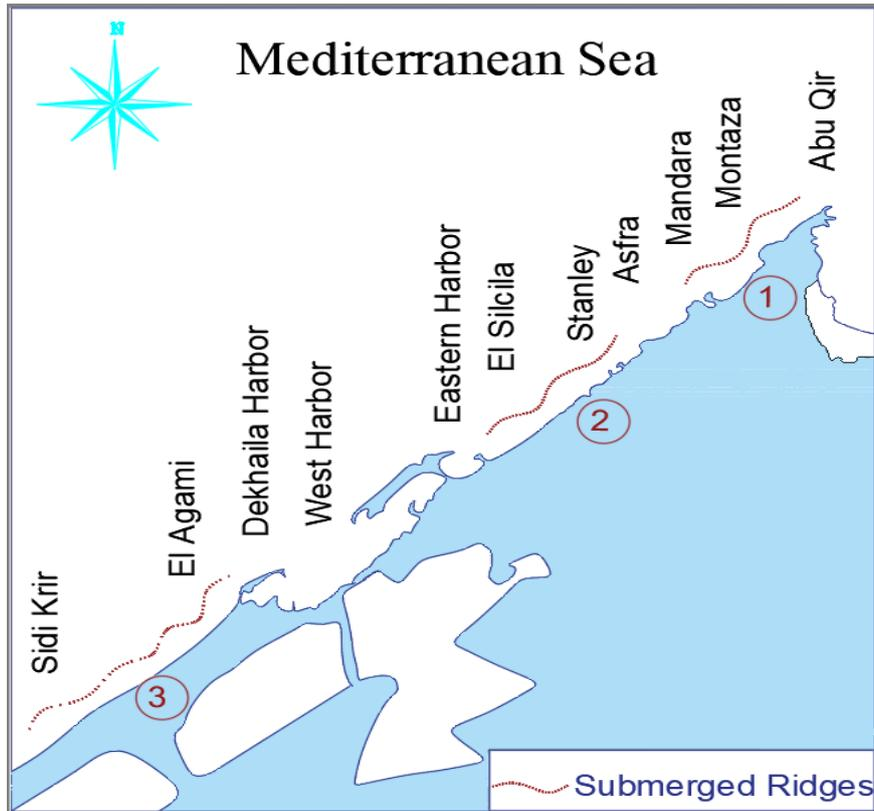
Figure 6: Submerged ridges located along the Alexandria coast distributed in three locations parallel (By Author)
