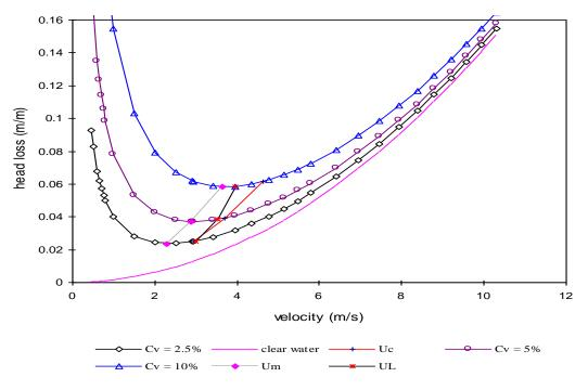
Fig (4): Head Loss Curves and Critical Velocities V<sub>m</sub>, V<sub>L</sub>, and V<sub>c</sub>
