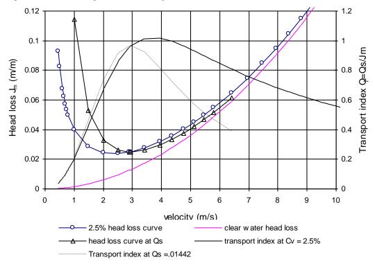
Fig (5): Head loss and transport index curves at constant C<sub>v</sub> and Q<sub>J</sub>
