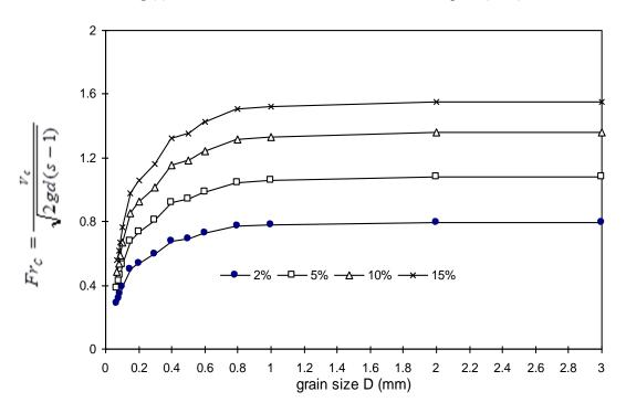
Fig (2): Computed Critical Durand Number Versus Sediment Grain Diameter with Concentration as Parameter
