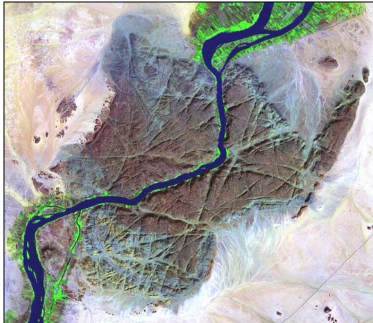
Figure 3: Colour composite of the Plateau obtained using bands 7, 4, 1 in RGB, respectively
