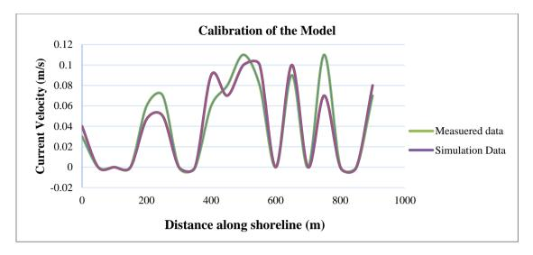
Figure 12: Calibration of Current Speed velocity (m/sec) Alexandria coast
