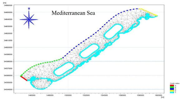
Figure 8: Mesh generation with external boundary condition and the new artificial islands (MIKE 21 Sw)
