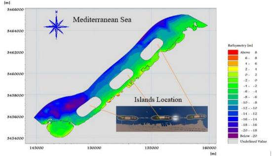
Figure 9: Generated bathymetry by using Mike21 showed the different depths at the artificial island location. The end of the Artificial Island reaches a depth of 10 m.
