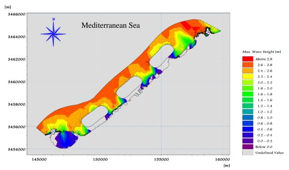
Figure 13: Wave distribution by the annual normal wave by max =2.85 m
